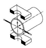
According to Faraday electromagnetism principte, the induced tension, in a conductor moving in a magnetic field, is directly proportional to the conductor speed.
