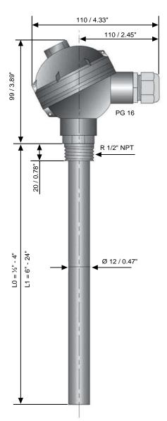
Industrial probes and boards are base on : Ro = 100 Ohms R 100°C = 138,5 Ohms
