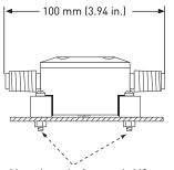
Mounting tabs for metric M3 or standard #6 screws on 68 mm (2.68 in.) bolt circle Side View
