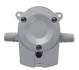
The Signet 2000 Micro Flow Rotor Sensor is constructed of Polyphenylene Sulfide (PPS) which provides high material strength. The 2000 offers two flow ranges starting at 0.11 or 1.13 lpm (0.03 or 0.3 gpm), for clean process liquids, regardless of fluid color or opacity.
